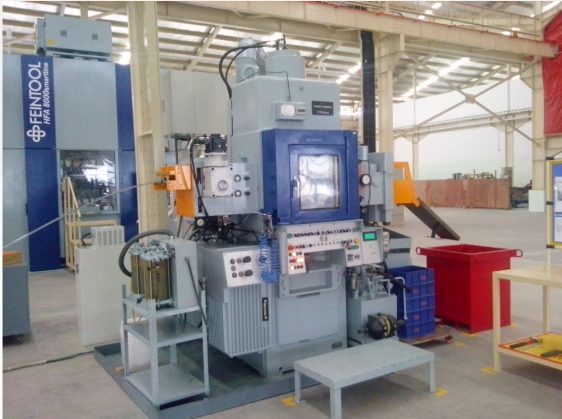
Fine Blanking 160T : max thickness 6 mm
