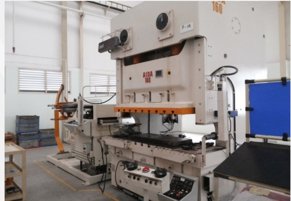
P160T with progressive : Max thick 3.2 mm
