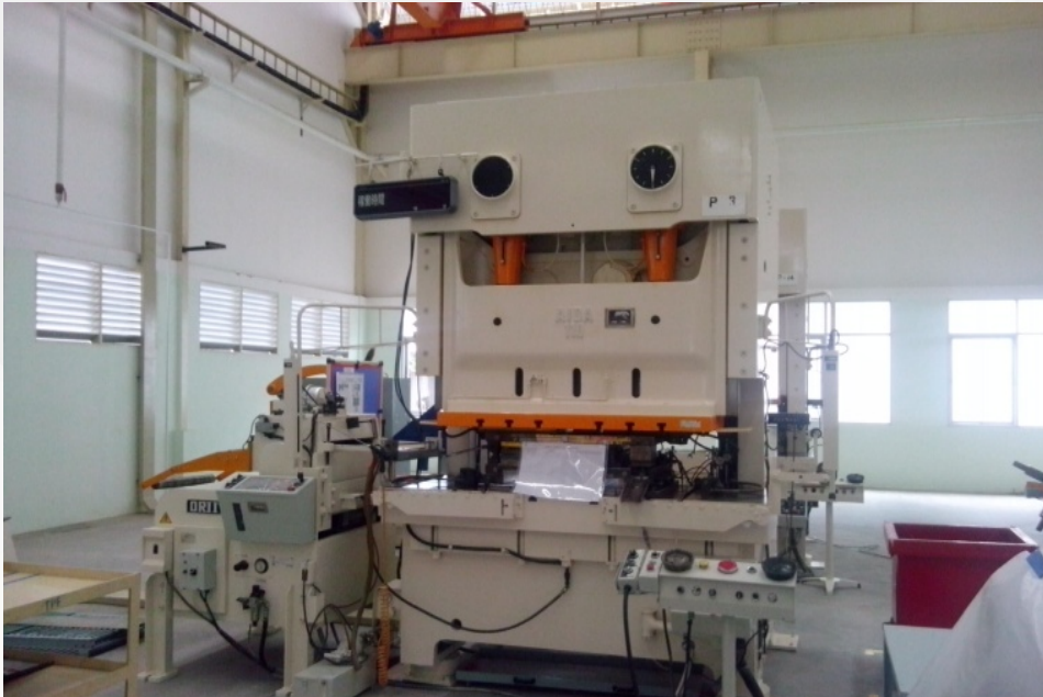
P110T with progressive : Max thick 3.2 mm
