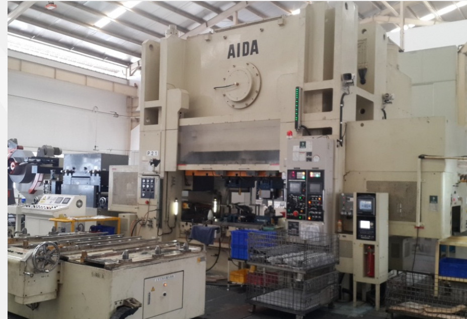
UL600T AIDA Max thick 8 mm, progressive 3D transfer
