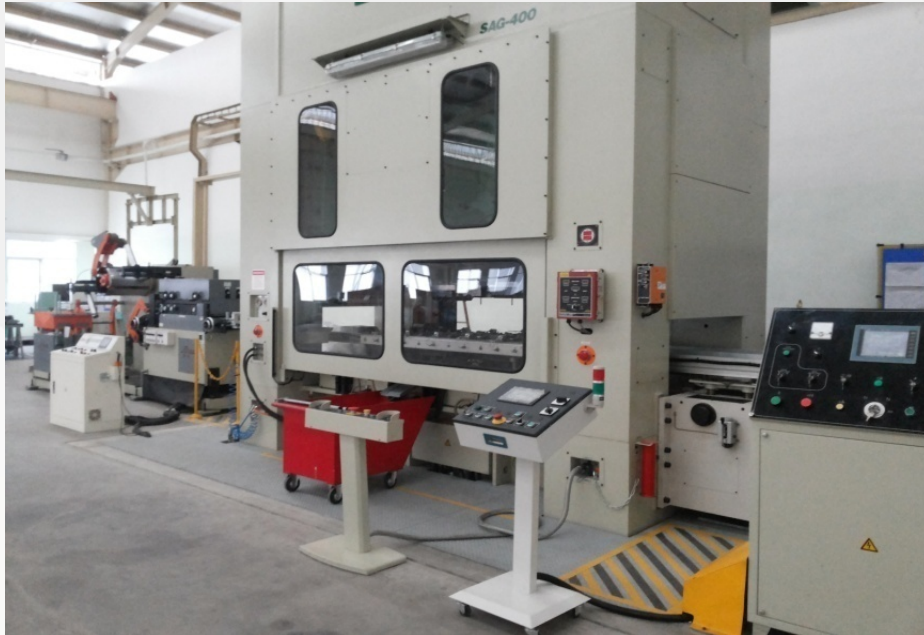
P400T with progressive and 3D transfer : Max thick 6 mm, deep stroke (max parts height 125 mm)
