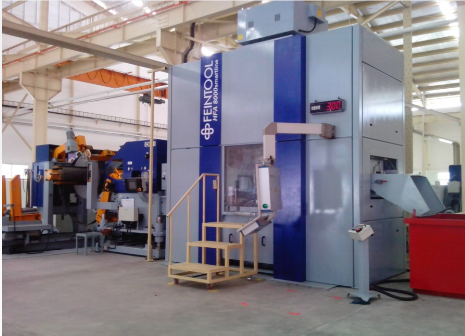
Fine Blanking 800T : max thickness 12 mm -Tandem and Progressive capability
